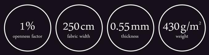
THIS FABRIC IS MADE FROM COATED FIBRE GLASS ACOUSTIC ABSORPTION FACTOR  $\mathcal{A}_{W}$  : 0.35 to 0.8
