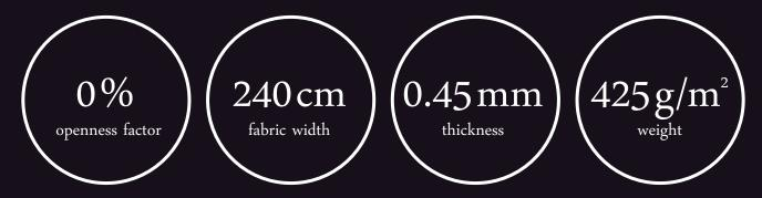
THIS FABRIC IS MADE FROM 100 % FIBRE GLASS
