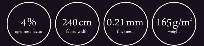
THIS FABRIC IS MADE FROM 100 % FIBRE GLASS
